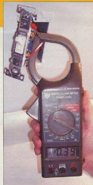
A tick tester is used to check power at switches.
